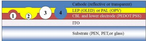
Fig. 1: Solution processed white OLED displaying visible colour and brightness inhomogeneity
